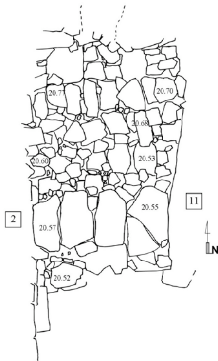
Fig. 20. Area A, Square 13. Sub-floor channel system of Phase AIII (Locus 33) beneath central part of Room 19, covering slabs still in situ. Scale 1:40.
